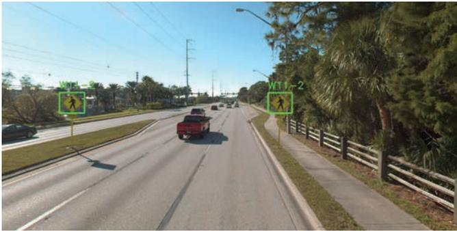
The traffic sign identification results can be delivered in various file formats including JavaScript Object Notation (JSON), Extensible Markup Language (XML), and Comma-Separated Values (CSV) format. The results include MUTCD sign types and localization information in the form of pixel coordinates against each detected sign with a confidence score. The confidence score can be used by
